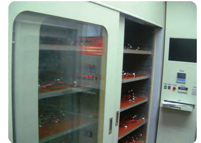
DC fan aging box and monitoring system
